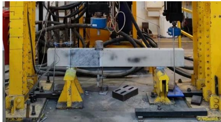
Figure 2. Three-point bending test set-up.
